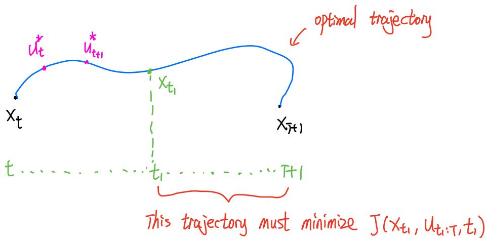
$$\begin{aligned} \min_{u_{t:T}} J(x_t, u_{t:T}, t) &= \sum_{s=t}^T L(x_s, u_s) + l(x_{T+1}) \\ &= \sum_{s=t}^{t_1} L(x_s, u_s) + \underbrace{\sum_{s=t_1}^T L(x_s, u_s) + l(x_{T+1})}_{J(x_{t_1}, u_{t_1:T}, t_1)} \end{aligned}$$
