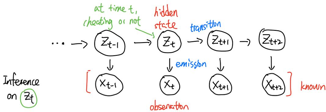
$$P(z_t | x_{1:T}) \propto P(z_t, x_{1:T}) = \underbrace{P(x_{1:t}, z_t)}_{\alpha_t(z_t) \text{ forward}} \underbrace{P(x_{t+1:T} | z_t)}_{\beta_t(z_t) \text{ backward}}$$
